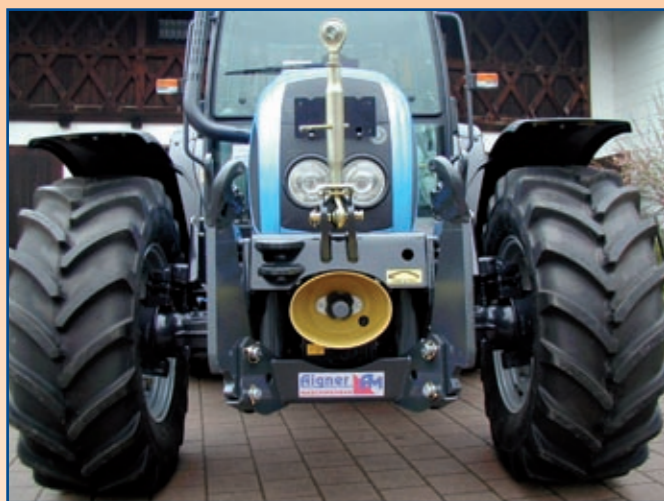
Lower links fold inward diagonally - optimum in case of the combination frontlinkage + front loaders!
