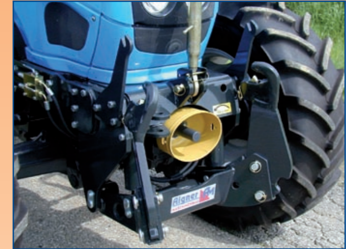
frontlinkage and PTO for a compact unit
