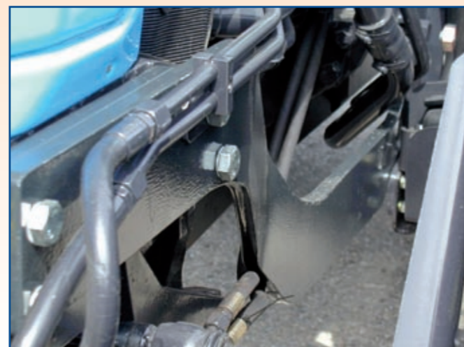
Stable frame up to clutch bell housing - Uninhibited front axle oscillation
