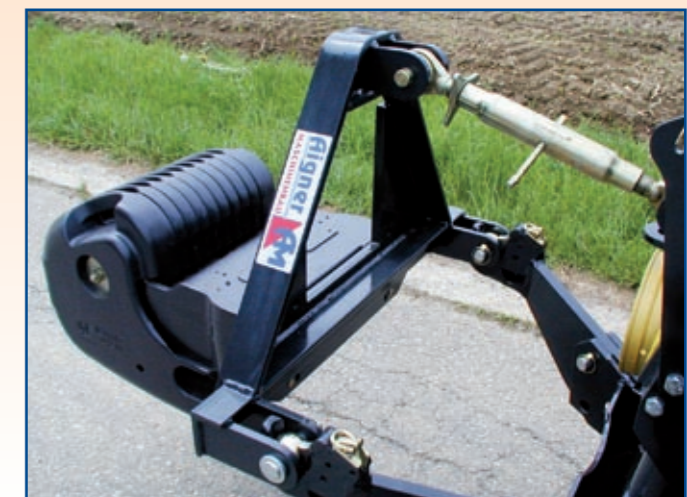
Attachment frame for tractor net weight 3-point attachment or for quick coupling triangle
